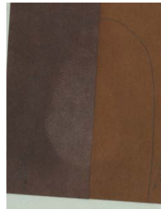
FIG. 5—The difference between the intensity of silver nitrate development between the irradiated (right) and control (left) samples.
