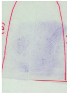
FIG. 11—An example of the minor differences between irradiated (right) and control (left) samples that have been treated with Gentian violet.
