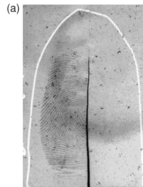
FIG. 8—Side effects of the irradiation process: a wrinkling effect present in the irradiated trash bag sample (left) (a) and the discoloration that occurred with the PVC samples (right) (b).
