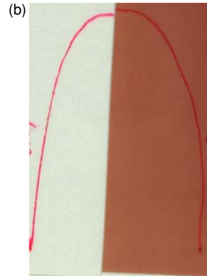
FIG. 8—Side effects of the irradiation process: a wrinkling effect present in the irradiated trash bag sample (left) (a) and the discoloration that occurred with the PVC samples (right) (b).
