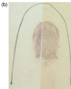
FIG. 7—A difference between the intensity and color of iodine development between the irradiated (left) and control (right) samples (a) and a similar example in which a difference in color and intensity can be seen between the irradiated (right) and control (left) samples (b).
